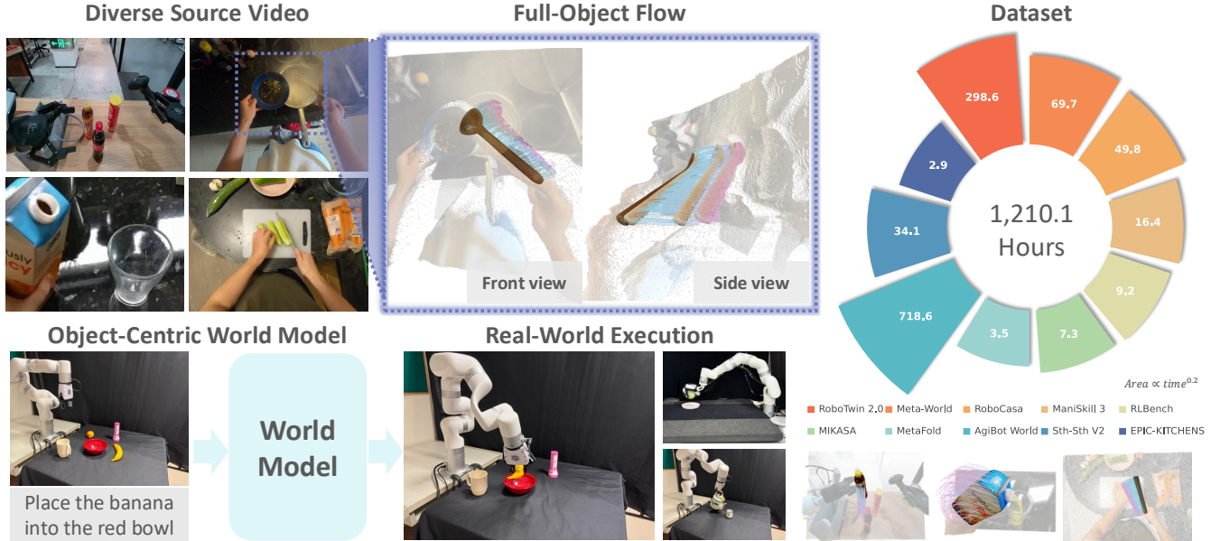
Fig. 1: From diverse videos to executable full-object flow. We construct a 1,210.1-hour dataset of 3D full-object flow from diverse real-world and simulated videos. An object-centric world model predicts dense motion over the complete object surface from image-and-language inputs, and the predicted flow guides downstream robot execution. The radial chart summarizes its composition across seven simulation datasets and three large-scale real-world video sources.
